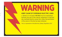
All Mobile cranes on a Ryman Healthcare Construction site must display 'Warning Keep Clear of Overhead Electric Lines' as required by the Electricity (Safety) Regulations 2010.
